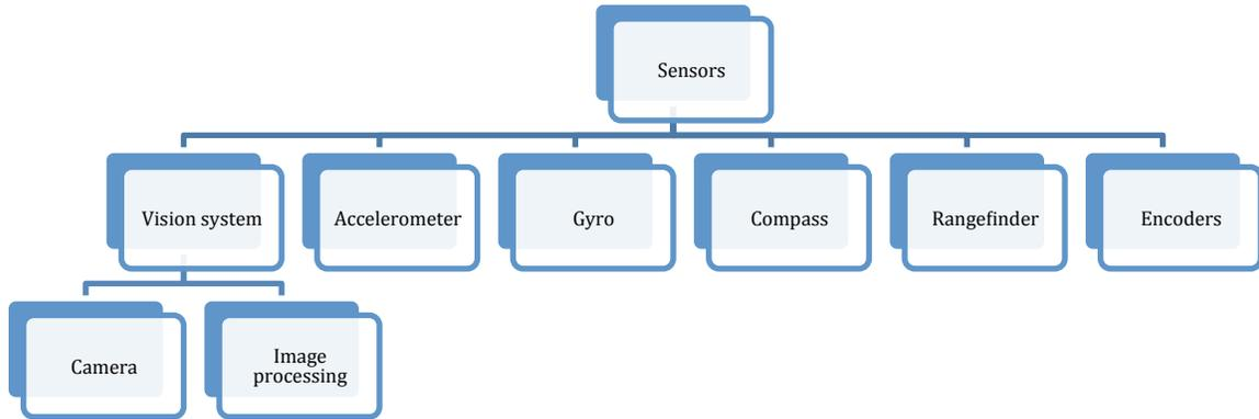
Figure 6: WPILib sensor section
